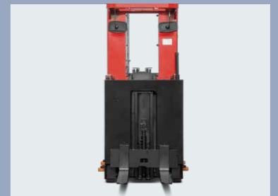
Supplementary lift on operator platform. Pallet can be raised to most convenient working level for picking
