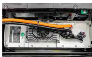
[Option] Lithium battery with the on-board charger (48V, 20A)
