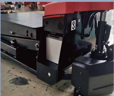
The batteries can be removed conveniently, for easier maintenance and disassembly
