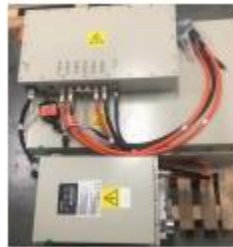
Orange high-voltage connection line
