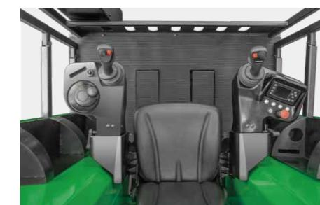
*The double safety pedals, left and right guardrails, automatic induction joystick and other active and passive safety systems are equipped to prevent hazards caused by mis-operation.*
