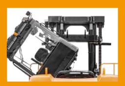
The over-turnable cab and electric tipping cylinde make tipping easier and more labor-saving.
