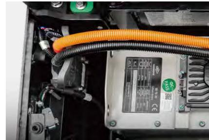
The power plug is fixed on the truck body to avoid damage from battery installment.
