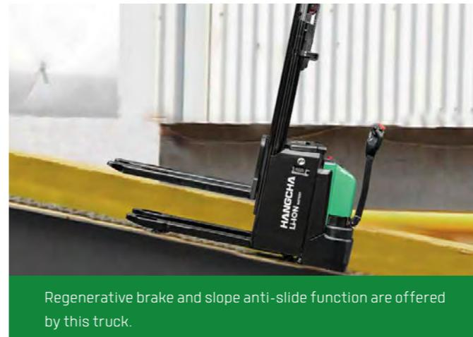
Regenerative brake and slope anti-slide function are offered by this truck.
