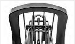
The truck with assembly overhead guard can protect the driver's safety in case of high-position cargo falling. (Rider Model)
