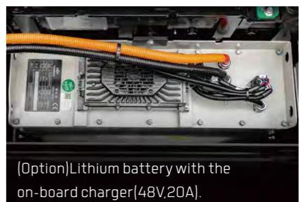
(Option)Lithium battery with the on-board charger(48V,20A).
