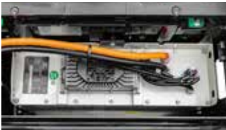
(Option)Lithium battery with the on-board charger(48V,20A)
